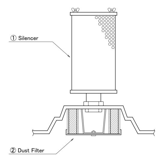
Please use the fine dust filter set for collecting fine dust/ powders, as this model is not designed for fine dust collection.
