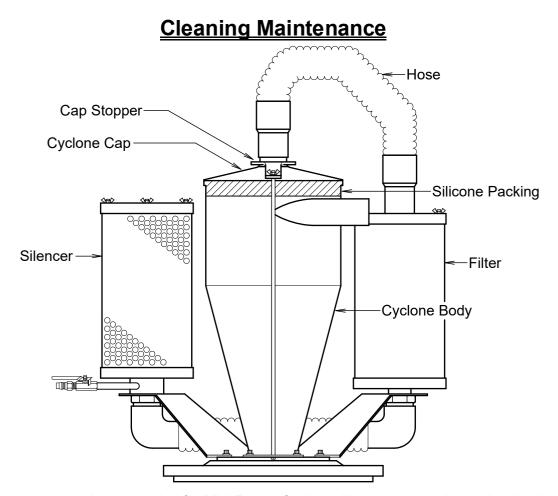
Frequent maintenance is not needed for Mini-Porter-Cyclone. However, occasional cleaning is required in the inside of the body to maintain optimal performance. To clean, brush the inside occasionally. Especially after vacuuming the moist dust, brush well or wipe well with the dry cloth since the moist dust stays inside.
