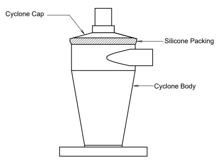
※ Frequent maintenance is not needed for Mini-Porter-Cyclone. However, occasional cleaning is required inside of the body to maintain optimal performance. To clean, brush the inside occasionally. Especially after vacuuming the moist dust, brush well or wipe well with the dry cloth since the moist dust stays inside.
